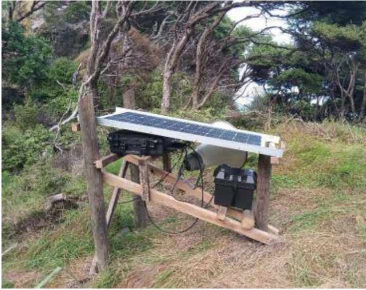
Seabird audio attraction station installed by ranger Clint Stannard, at the head of Taraire Valley on the southwestern side of the island, one speaker facing towards Hauturu & the other down the valley. Photo: Clint Stannard.
